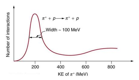
Figure 2: The probability of the interaction between a  $\pi^+$  and a proton as a function of the kinetic  $\pi$  energy.
