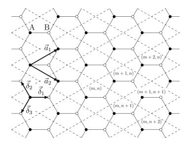
Figure 1: Graphene lattice
