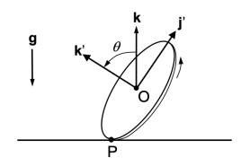
a. The condition of perfect rolling means that the velocity in contact point P is zero. Use this to show that
