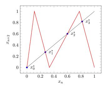
Figure 3: Skewed tent map, second iterate. As the tent has its apex at 1/3, the second iterate consists of a (compressed) copy between 0 and 1/3, and an inverted (compressed) copy between 1/3 and 1. The fixed points are 0, 3/7, 3/5, and 9/11. The slopes of the segments are 9, -9/2, 9/4, and -9/2; therefore all fixed points, again, are unstable.
