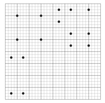
2. Now we want to apply the BSP tree approach for space partitioning to the same scene. Draw the resulting cells into the image below. Start with a vertical split and then alternate between horizontal and vertical splits. Stop once each cell contains a maximum of two objects.
