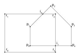
Draw the related graph that is used by the Weiler-Atherton algorithm for clipping arbitrary polygones. Start with vertices  $p_0$  and  $r_0$  and proceed in clockwise order (i.e. start with  $p_0$  and  $r_0$ , then  $p_1$  and  $r_1$ , and so on). Don't forget to clearly indicate which nodes are outgoing and incoming intersections.
