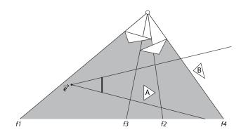
We want to render the scene on the screen (indicated by the bold line) towards the direction of our camera (indicated by the vector  $\vec{e}$ ). To check if the triangles A and B are in the shadow or not, we are using a Stencil Buffer.
